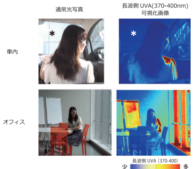
Fig. 5 In situ imaging of long wavelength UVA (370-400 nm) inside a car near the window
