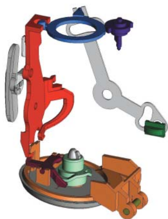
Fig. 8 Safety lock mechanism.
