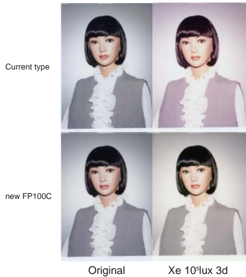
Photo 3 Comparison of new FP100C with the current type in image permanence.
