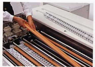
Photo 4 Cross-over part of the processor.
