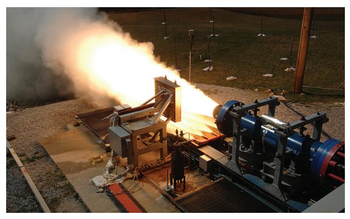
Marshall tested a small solid rocket motor designed to mimic NASA's SLS booster. The test provided an effective way to evaluate a new nozzle insulation material.
