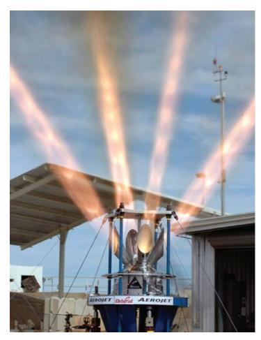
The successful test firing of the Orion jettison motor is the first full-scale rocket propulsion element qualified to proceed into a system-level demonstration.
