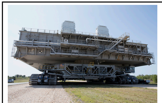
NASA's upgraded crawler-transporter 2 (CT-2), carrying mobile launcher platform 1, moves slowly along the crawlerway at KSC. The crawler's upgrades and modifications will be monitored and tested to confirm it is ready to support the load of the mobile launcher carrying the SLS with Orion atop for EM-1.
