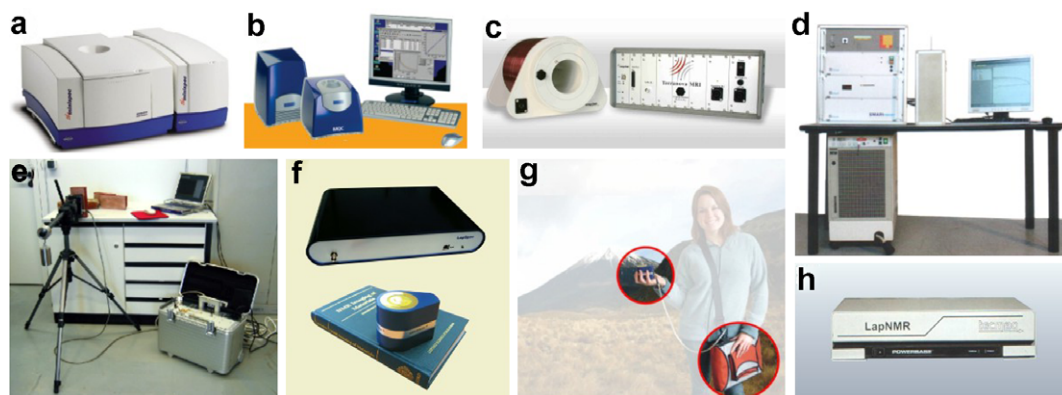
Fig. 14. Spectrometers for desk-top use and mobile NMR. (a) Bruker Minispec spectrometer and magnet (on left hand side) [252]. The spectrometer has variable frequency and can be used together with other NMR sensors like the NMR-MOUSE® [255] or the Bruker Profiler. (b) MQC desk-top instrument by Oxford Instruments consisting of a magnet and a spectrometer which includes the PC [253]. (c) Low-cost earth-field NMR spectrometer Terranova by Magritek, Wellington, New Zealand [257]. (d) Desk-top field cycling spectrometer SMARtracer by Stelar, designed to measure relaxation times as a function of field strength [258]. (e) NMR-MOUSE mounted on a tripod and Bruker Minispec console in a pilot's aluminum travelling case by RWTH Aachen University [259]. (f) Variable frequency spectrometer LapSpec for mobile NMR by ACT GmbH, Roetgen [260] and Magritek [257] together with the Easy NMR-MOUSE® [188]. (g) Lap-top size variable frequency NMR spectrometer with a battery pack for out-door's operation by Magritek [257] and ACT GmbH [260] and Easy NMR-MOUSE. (h) Variable frequency NMR spectrometer LapNMR by Tecmag [261].
