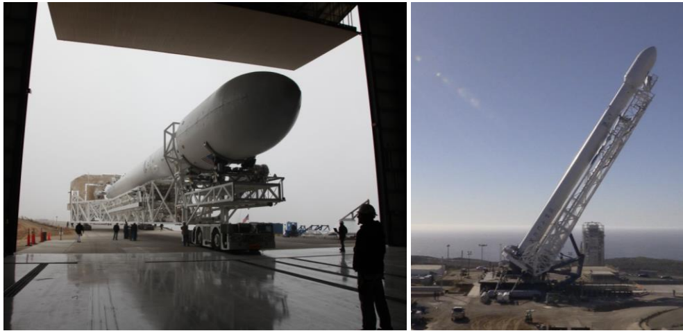
Figure 8-8: Launch vehicle rollout and erection
