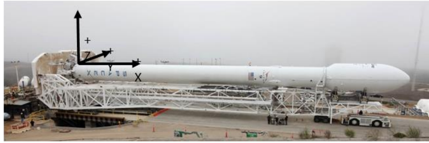
Figure 2-2: Falcon vehicle coordinate frame
