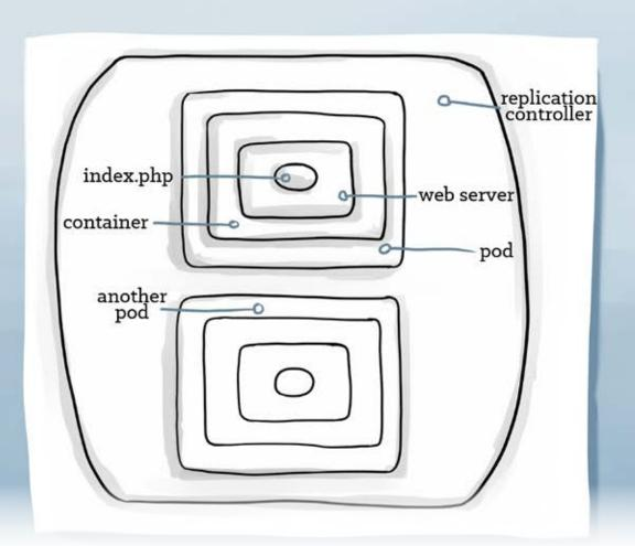
Replication controllers provide a method for managing an arbitrary number of pods. A replication controller contains a pod template, which can be replicated any number of times. Through the replication controller, Kubernetes will manage your pods' lifecycle, including scaling up and down, rolling deployments, and monitoring.
