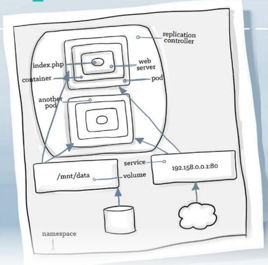
A namespace functions as a grouping mechanism inside of Kubernetes. Services, pods, replication controllers, and volumes can easily cooperate within a namespace, and the namespace provides a degree of isolation from other parts of the cluster.
