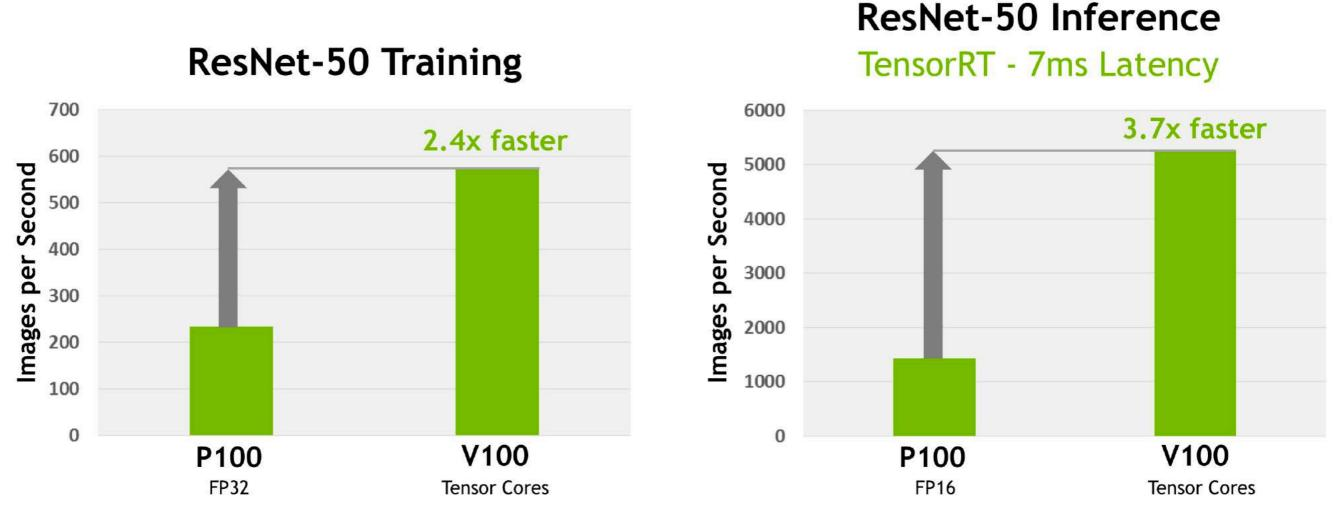
Left: Tesla V100 trains the ResNet-50 deep neural network 2.4x faster than Tesla P100. Right: Given a target latency per image of 7ms, Tesla V100 is able to perform inference using the ResNet-50 deep neural network 3.7x faster than Tesla P100.
