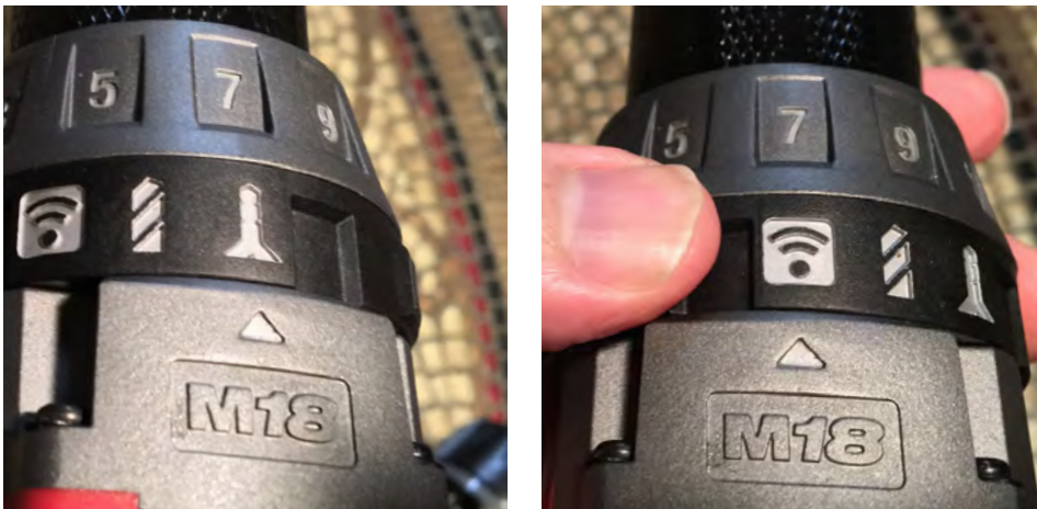
Normal usage on the left, Bluetooth profile update mode on the right.
