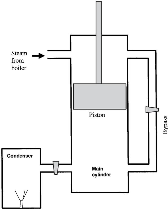
FIGURE 4.5. A diagram illustrating the workings of a Watt engine, adapted from Cardwell 1971, 49, and Sandfort 1964, 31. Hot steam enters the upper part of the main cylinder, pushing down the piston and performing work; then the piston is pulled back up; at the same time the bypass valve is opened to allow the steam to pass to the part of the cylinder below the piston; from there it gets sucked into the condenser, where a jet of cold water cools it and turns it into liquid water.
