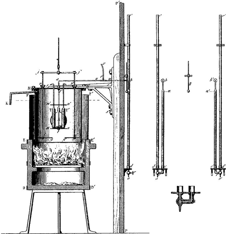
FIGURE 2.2. Regnault's constant-volume air thermometer, illustration from Regnault 1847, 168–171, figs. 13 and 14. Courtesy of the British Library.
