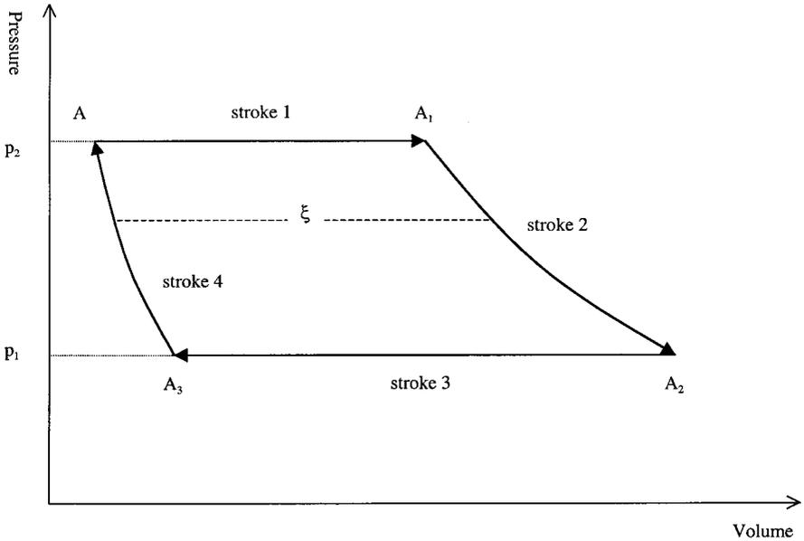
FIGURE 4.8. The indicator-diagram representation of the working of the ideal steam-water cycle, adapted from Thomson [1849] 1882, 124.
