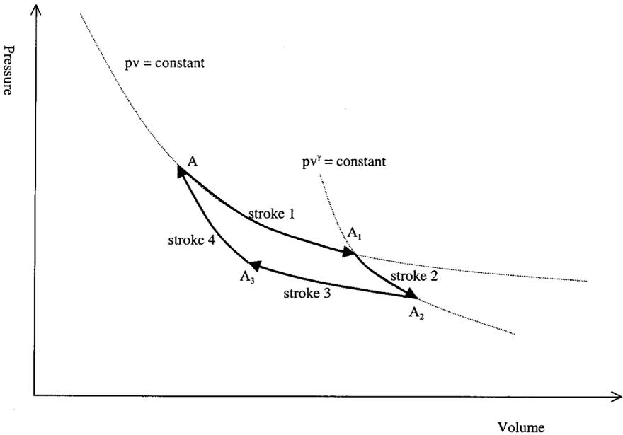
FIGURE 4.7. The indicator-diagram representation of the Carnot cycle, for the case of an air engine, adapted from Clapeyron [1834] 1837, 350.
