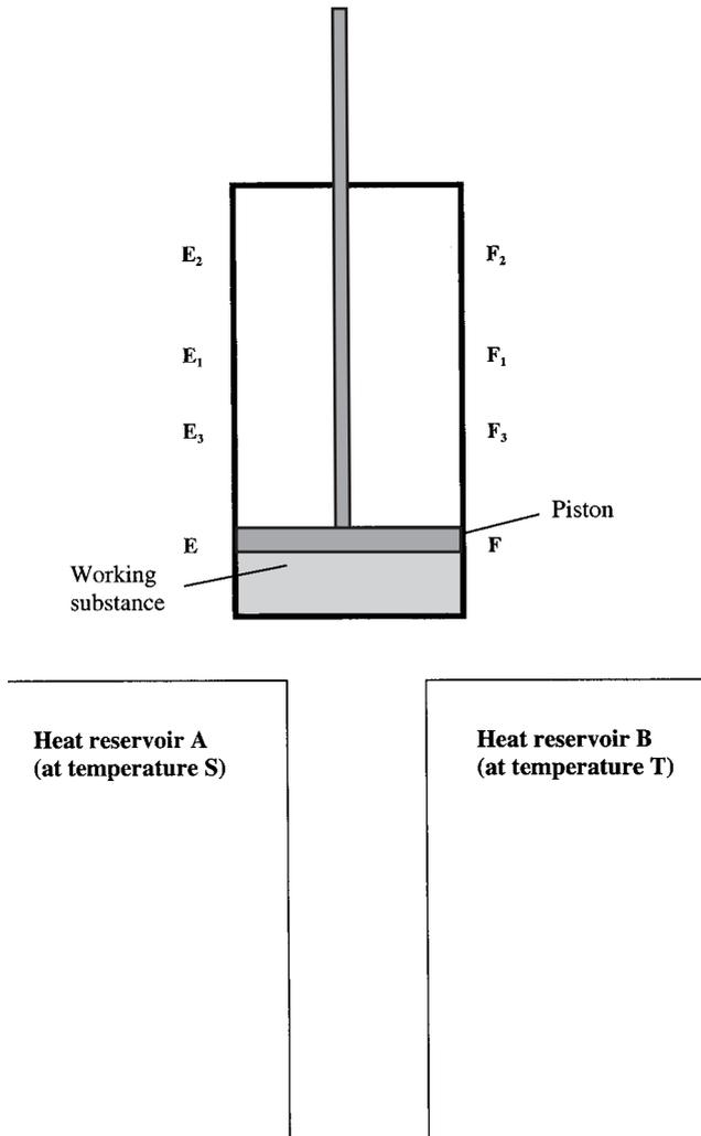
FIGURE 4.6. A schematic representation of a possible form of the Carnot engine, adapted from Thomson [1849] 1882, 121.
