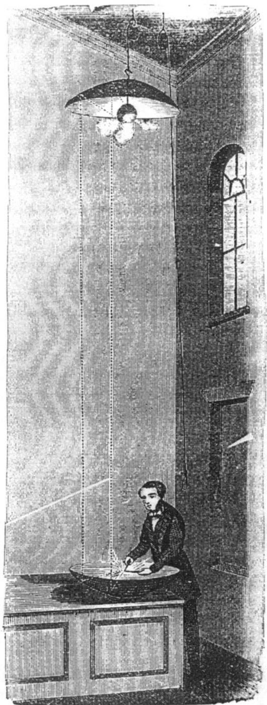
FIGURE 4.3. Illustration showing a version of Pictet's "double-reflection" experiment, from Tyndall 1880 (290). The spark ignited at the focus of the lower mirror causes the explosion of the hydrogen-chlorine balloon at the focus of the upper mirror. In an experiment more like Pictet's, a hot copper ball placed in the lower focus causes a blackened hydrogen-oxygen balloon at the upper focus to explode. Courtesy of the British Library.
