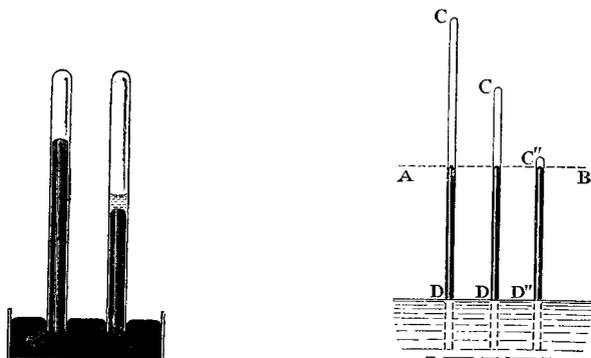
FIGURE 1.4. Experiments illustrating the pressure of saturated vapor (Preston 1904, 395).
