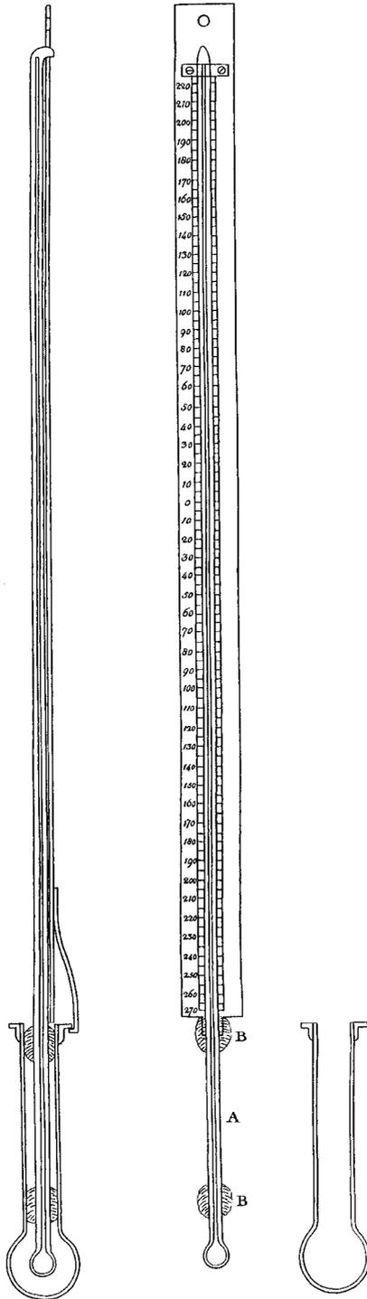
FIGURE 3.2. Cavendish's apparatus for determining the freezing point of mercury, used by Hutchins (1783, tab. 7, facing p. \*370). Courtesy of the British Library.
