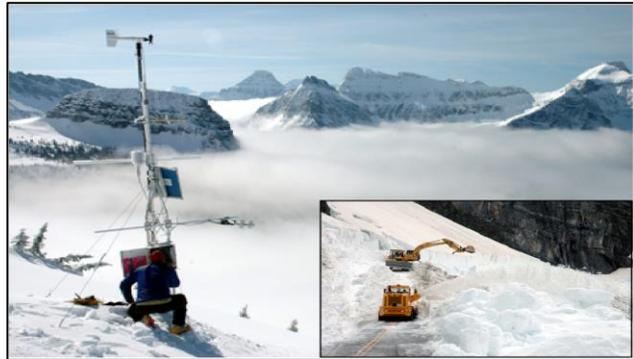
**By combining analysis of meteorological data (such as information obtained from the Garden Wall weather station at 7,400 ft. in Glacier National Park, Montana) and measurements of snowpack depth, structure and water content, USGS researchers are improving avalanche forecasting in the park. This provides real-time snow safety and weather data to aid snow removal operations and recreational use of the park.**
