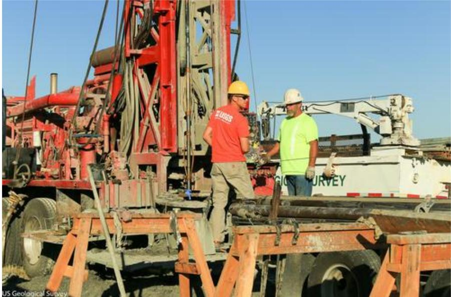
**Figure 7: USGS scientists drilling a research core near Waco, Texas. This core was drilled by USGS during field work for an oil and gas assessment for the Eagle Ford of the Gulf Coast Basins. Cores like these provide information on the various rock layers, such as their make-up, age, etc. Source: USGS ERP.**
