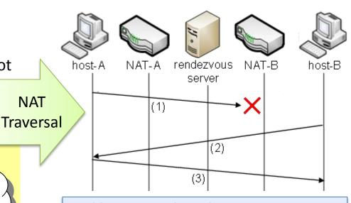
End hosts can directly communicate each other beyond NATs by using the UDP Hole Punching. However, they can traverse the only Cone NAT [RFC3489] i.e., cannot traverse a Symmetric NAT.
