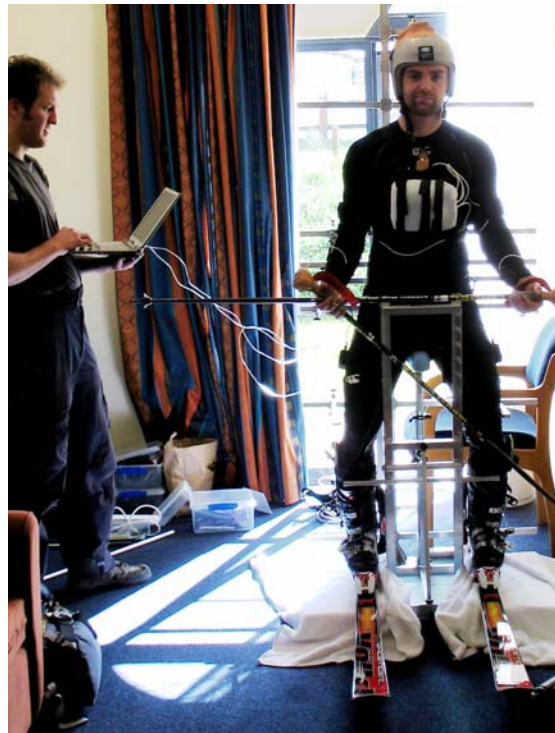
Figure 2.7: Mapping the local IMU coordinate systems to the local body segments
