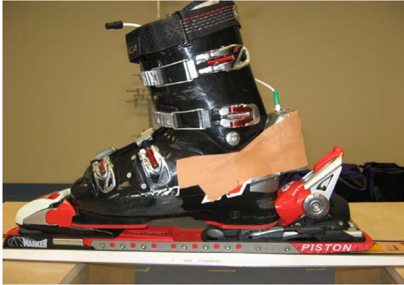
Figure 2.6: IMU placement behind the ski boot, in a waterproof protective casing.
