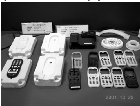
Figure-3. Injection molding die of TSR-2081 and its injected ABS product.
