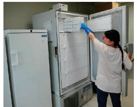
DNA・組織標本を保存する超低温冷凍庫 Ultra deep freezer which stores DNA and tissue specimens
