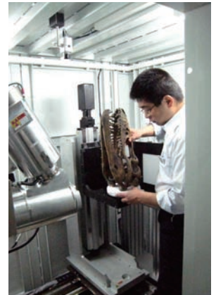
脊椎動物化石のX線CTスキャン A vertebrate fossil being set up for the X-ray computed tomography scan
