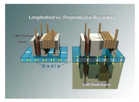
Seagate has demonstrated a recording areal density with perpendicular recording of 245 Gbpsi (Gigabits per square inch) with a data rate of 480 Mbits per second—more than double the 110 Gbpsi used in today's highest areal density disc drives—and 500 Gbpsi, which will increase the capacity of today's drives five-fold, is possible with the new technology.
