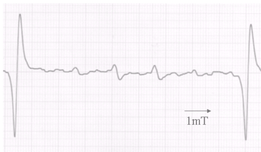
Figure 6 Test repeated with the addition of sulfuric acid to the water. The spectrum changed to that of DMPO-OH, indicating the production of ·OH.
