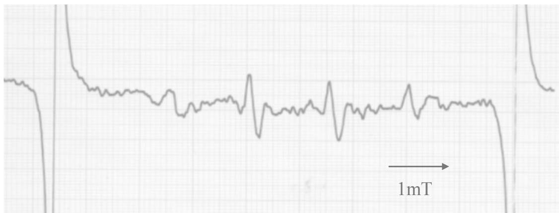
Figure 2. ESR spectrum of distilled water sample containing ozone macrobubbles and DMPO taken 20 s after bubbling had started. The spectrum indicates the presence of DMPO-OH, pointing to the production of hydroxyl radicals. The same level of DMPO-OH was observed with the addition of HCl.
