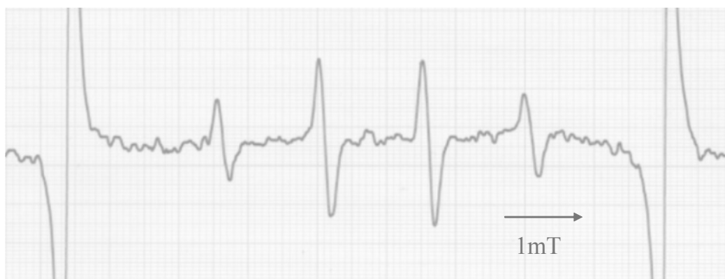
Figure 4. ESR spectrum of sample containing ozone microbubbles and DMPO with the addition of HCl, taken 5 s after bubbling had started. The spectrum shows that more hydroxyl radicals were generated under these strongly acidic conditions.
