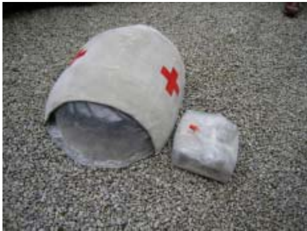
Figure 5: Concrete Canvas- a rapidly deployable concrete shelter (Brewin and Crawford, Ref.11)
