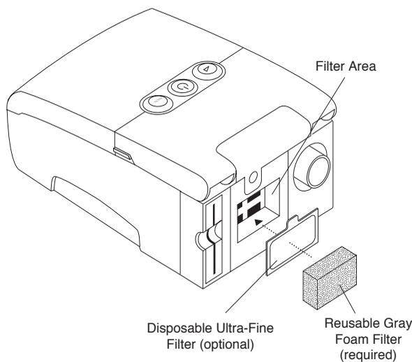
**FIGURE 3-1 INSTALLING THE AIR FILTER**
