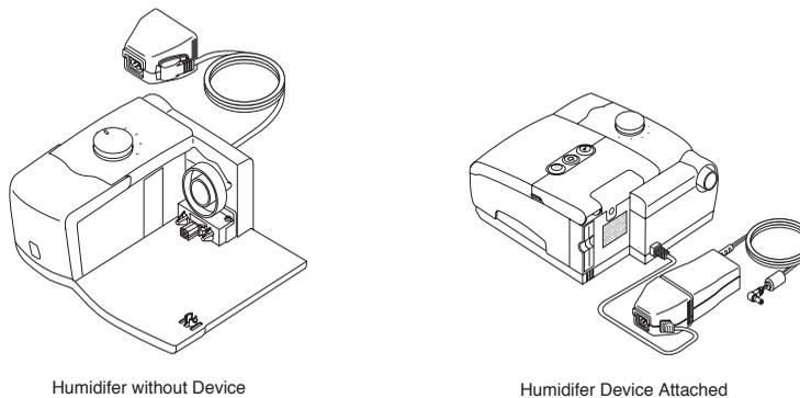
**FIGURE 6–1 HUMIDIFIER ALONE AND ATTACHED TO THE DEVICE**
