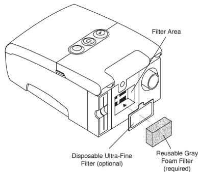
**FIGURE 7-2 REINSTALLING THE FILTERS**
