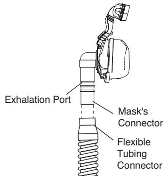
**FIGURE 3-3 CONNECTING A MASK WITH BUILT-IN EXHALATION PORT**
