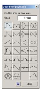
**Tip:** You can modify door swings very easily: activate the **Door** tool and click in the door opening. Select a different door swing in the dialog box that appears. The old one is deleted automatically.
