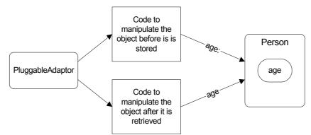
Figure 24-9. The PluggableAdaptor mechanism.
