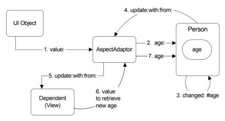
Figure 24-4. The AspectAdaptor mechanism.
