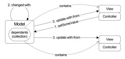
Figure 23-2. Model-View-Controller interactions.
