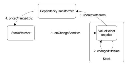
Figure 19-3. The addDependent: mechanism.
