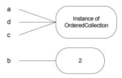
Figure 4-2. Variables holding different objects.
