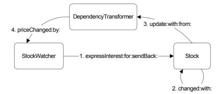
Figure 19-2. The addDependent: mechanism.
